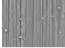
Ra=0.078μm GS-mill (Smooth surface !)
