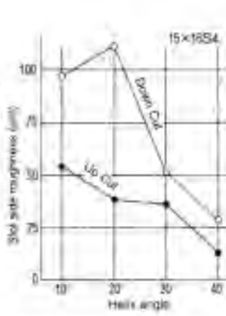
Relation between Helix angle and Slot side roughness
